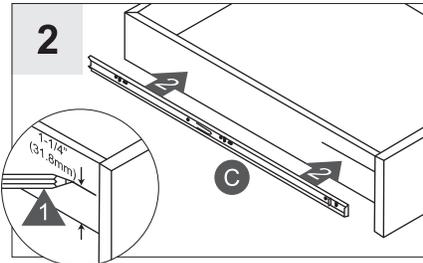
Mark 1-1/4" (32mm) from the bottom of the drawer side panel. Align the top of the drawer member (C) with mark.
