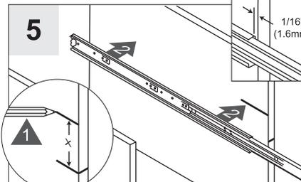
Mark "X" from the bottom of the mark. Repeat Step #1 to remove drawer member (C) from the Cabinet member (A). Align top of the cabinet member (A) with the mark, 1/16" from the front of the cabinet.
