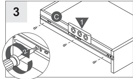
Make sure the drawer member (C) is level. Secure with screws. Repeat Steps 1-3 for the remaining drawer member.
