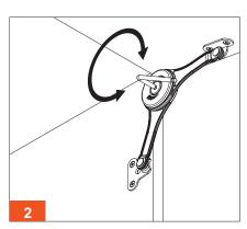
Adjust with allen key friction force according to flap door according to flap door dimension and weight using the adjusting screw.
