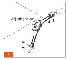
Fix always the brake leaving the adjusting screw always inside the cabinet.
