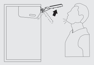
Use care when pulling out the lever. The lever may spring upward unexpectedly, potentially causing injury or damaging the lift system.!
