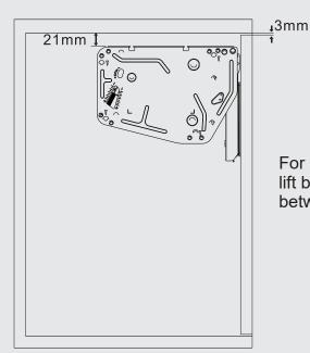
For inset applications, lower the lift by 21 mm to avoid interference between the door and the cabinet.
