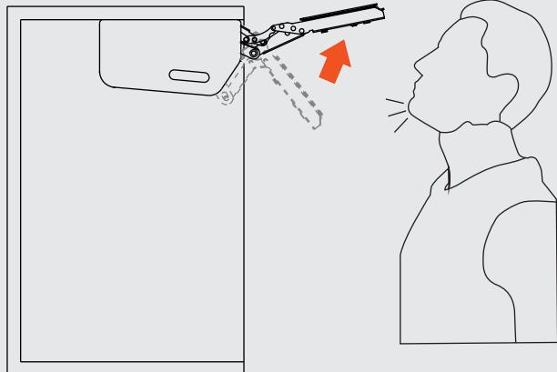
Use care when pulling out the lever. The lever may spring upward unexpectedly, potentially causing injury or damaging the lift system.!
