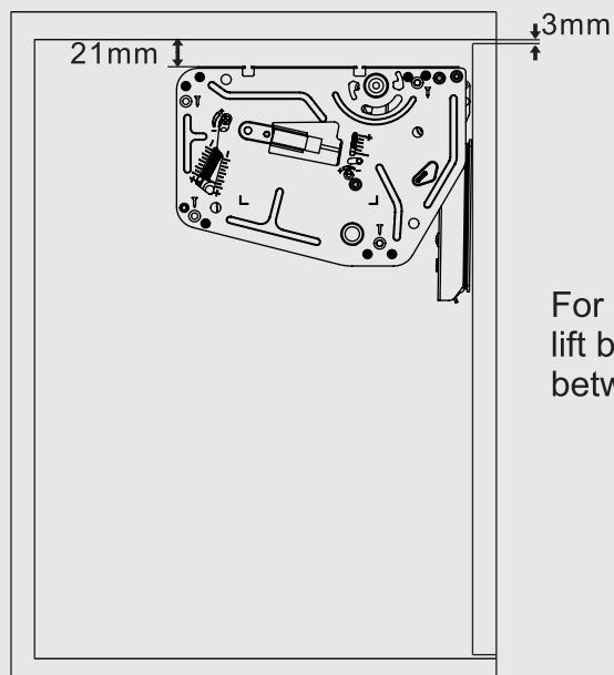
For inset applications, lower the lift by 21 mm to avoid interference between the door and the cabinet.
